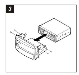
Slide the head unit into the *Radio Housing*, align the holes in the head unit with the holes in the Housing and mount the unit with the screws supplied with the unit.
